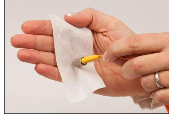
When cleaning connectors, the primary concern is the polished face. The face is the mating surface that comes into direct contact with another connector or the lens of an optical laser or detector. Any debris or residue on the connector face can have negative effect on the amount of signal that the connector is able to pass.
